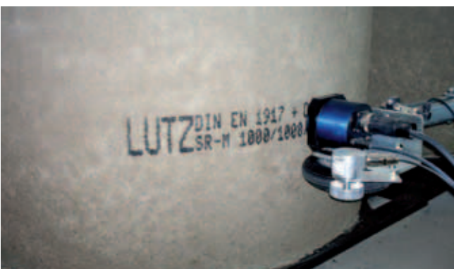
Marking of precast concrete pipes
