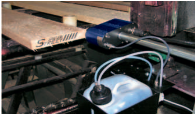
Marking on rough sawn timber boards
