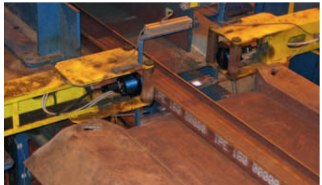
Marking of H-beams
