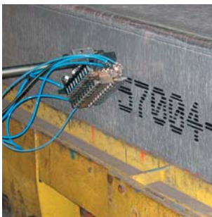
Alphanumeric marking of aluminum bars
