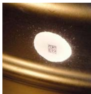
Mirror application for 2D DataMatrix Code
