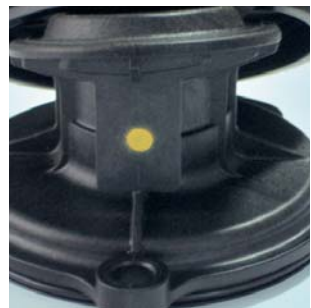
Marking of good parts after quality inspection
